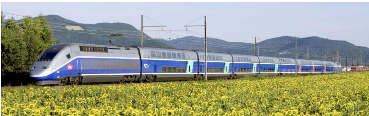
The TGV Duplex was introduced in 1995 as way to increase capacity on busy corridors. It features bi-level cars that can carry nearly 50% more passengers than single level trains.
